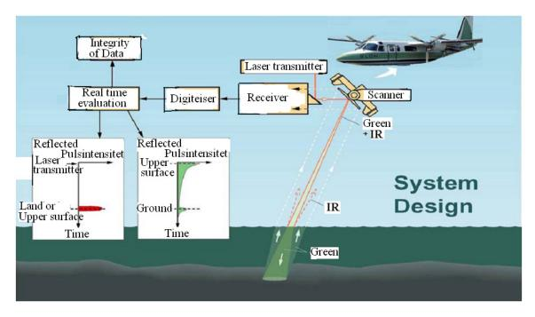
Fig.10. System for simultaneous scanning of underwater topography and land BLOM]
