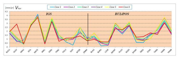
Fig. 7: Comparison of the horizontal velocities of the IGS and BULiPOS stations in ETRF2000
