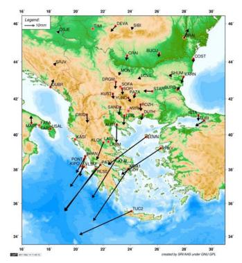
Fig. 3. Balkan Peninsula horizontal velocities with respect to stable Eurasia (after Stangl, 2011)
